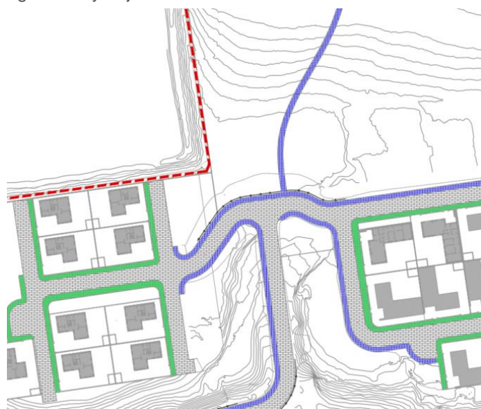
Figure 2-1 – Junction layout without road markings
