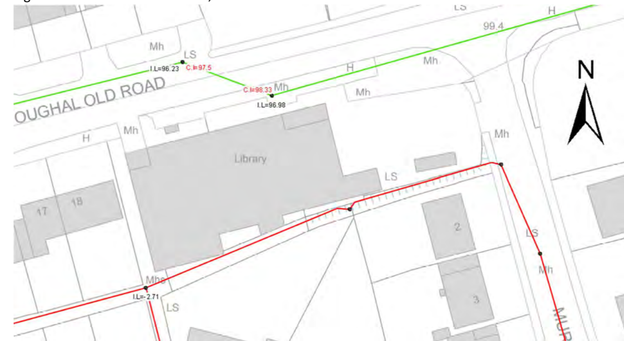
Figure 9- GREEN: combined drain, RED: foul drain
