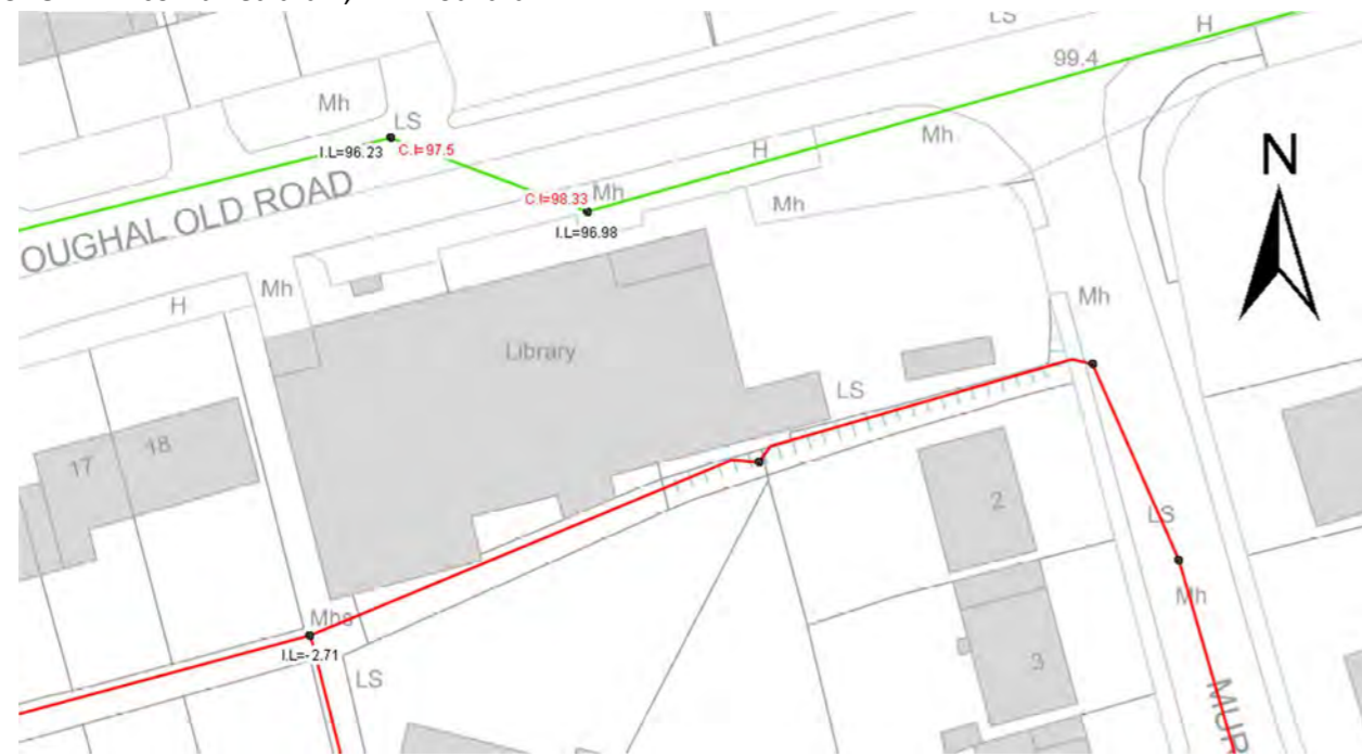
Figure 3- GREEN: combined drain, RED: foul drain
