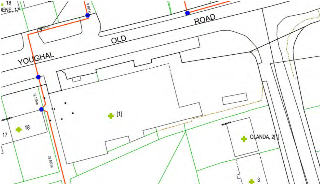
Figure 6 -Virgin Media cables
