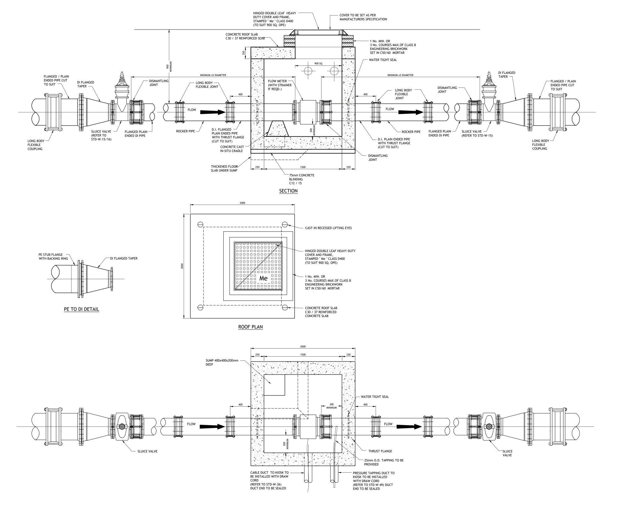
**FLOOR PLAN** METER CHAMBER (<=300mm DIA.)
