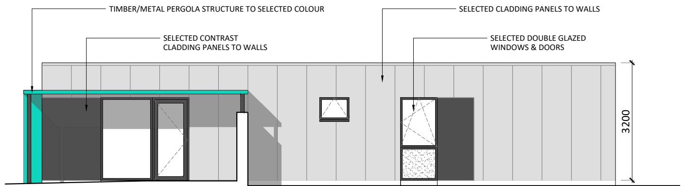
Type 2B: 1-bedroom accessible permanent modular unit adapted from Type 2A Side Elevation
