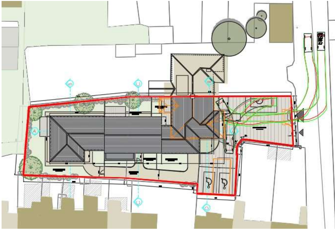
Fig. 21a: Turning analysis of the proposed parking space 1.
