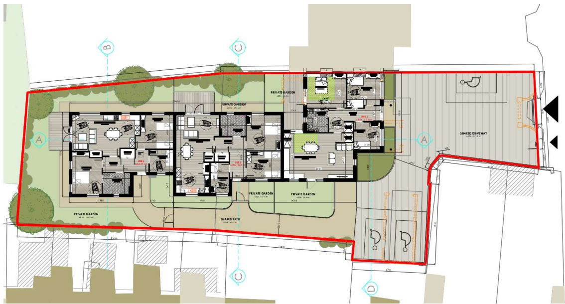
Fig. 24 : Proposed Site Layout by author showing the proposed dwellings & their relationship to the existing bungalow.
