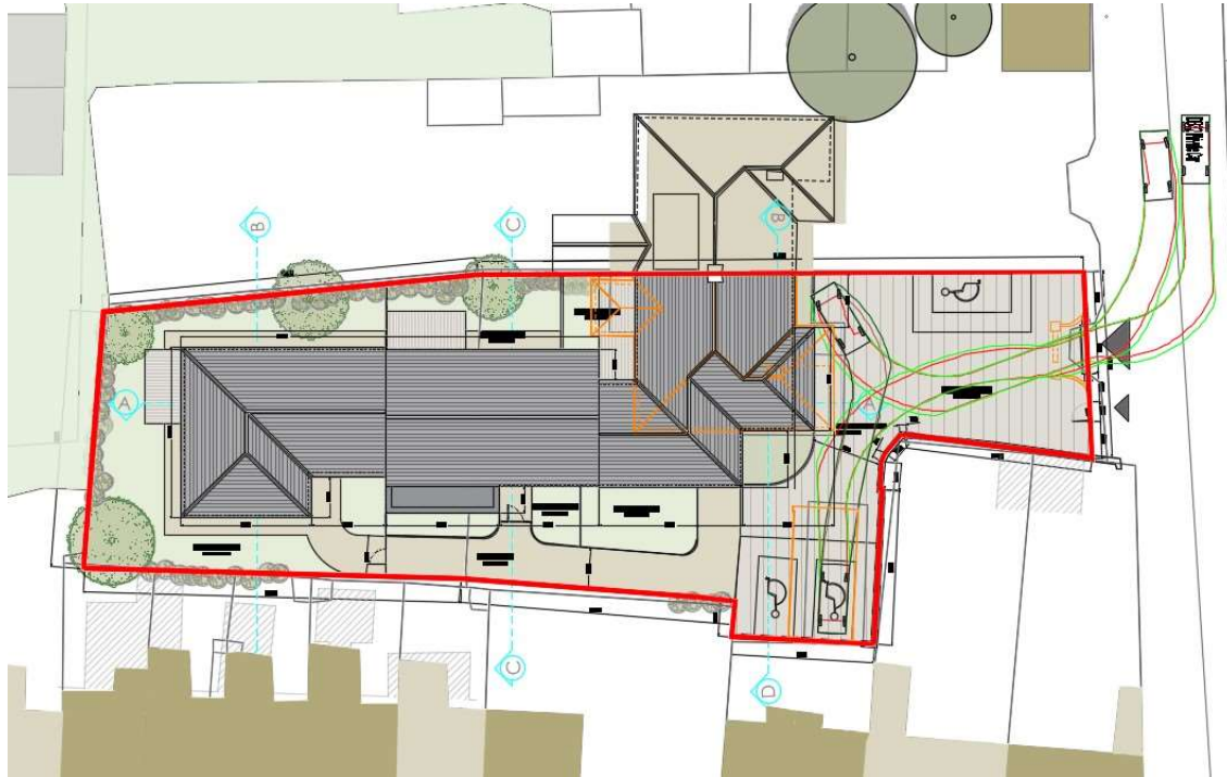
Fig. 21c: Turning analysis of the proposed parking space 3.
