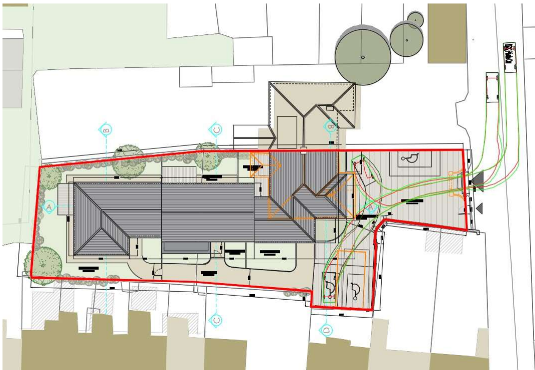
Fig. 21b: Turning analysis of the proposed parking space 2.
