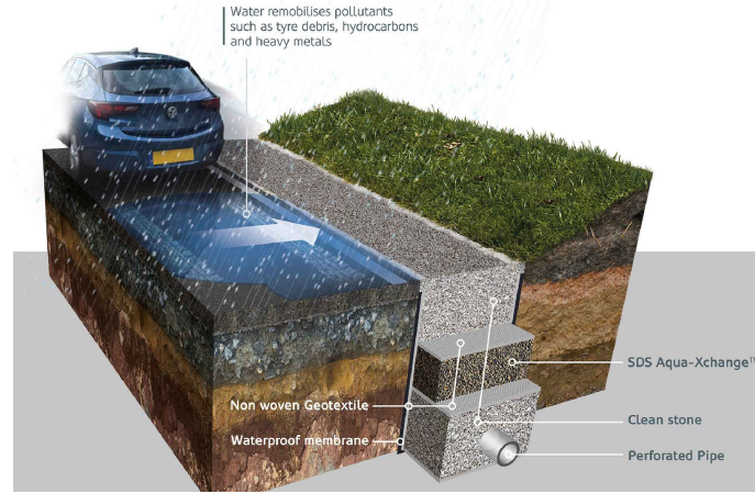
Typical Filter Drain Detail
