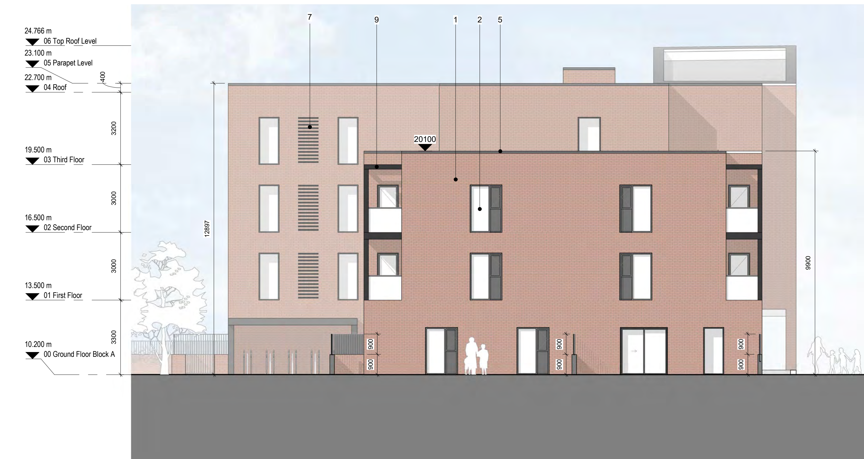
4 EAST ELEVATION BLOCK A 1 : 100
