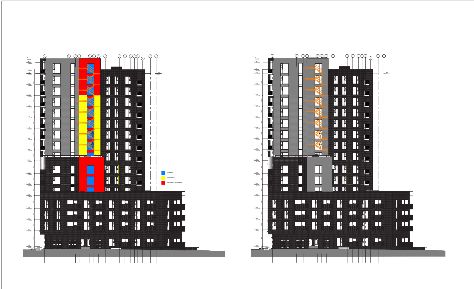
West Elevation Option 1 - Linear windows aligned with the adjacent windows for continuity & rhythm
