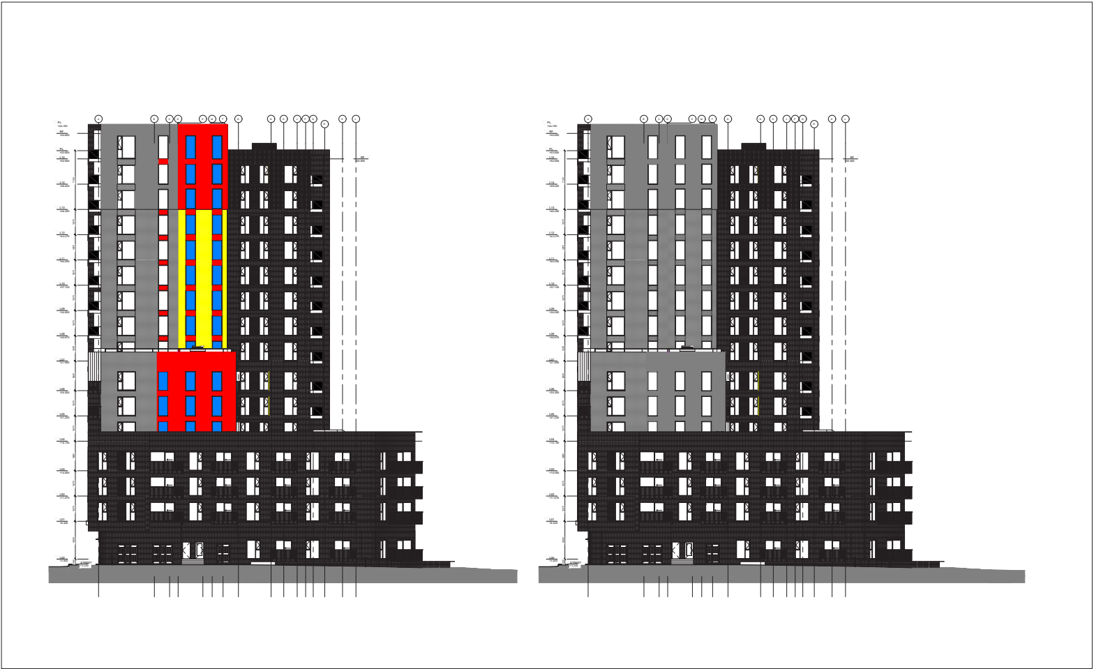
West Elevation Option 4 - Two linear rows of windows aligned with the adjacent facade for continuity.
