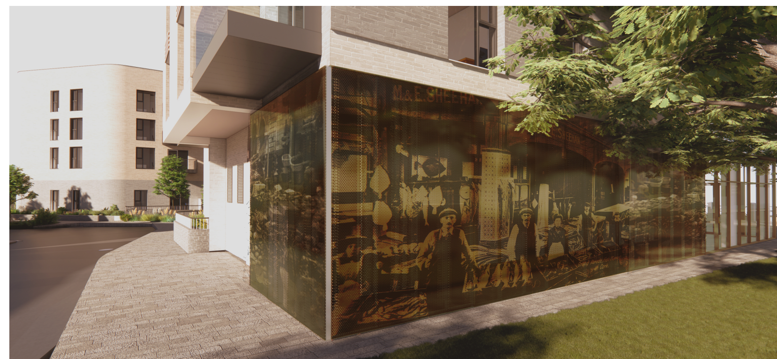
Bin Store - Indicative image of perforated metal screen with printed graphic (Image is indicative only)
