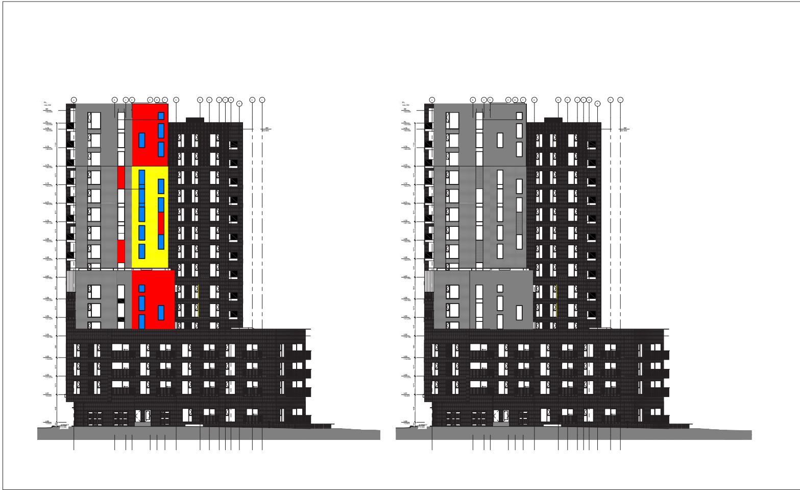
West Elevation Option 3 - Two staggered rows of thinner linear windows at varying heights, with spandrel panels, creating a less formal and more interesting composition.
