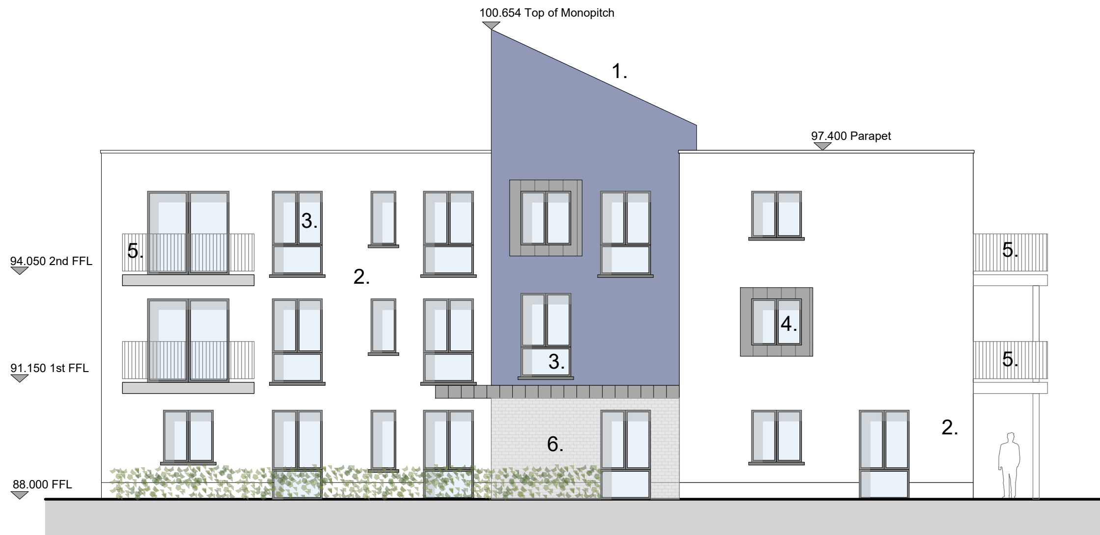
WEST ELEVATION - BLOCK D SCALE 1:100 (A3)
