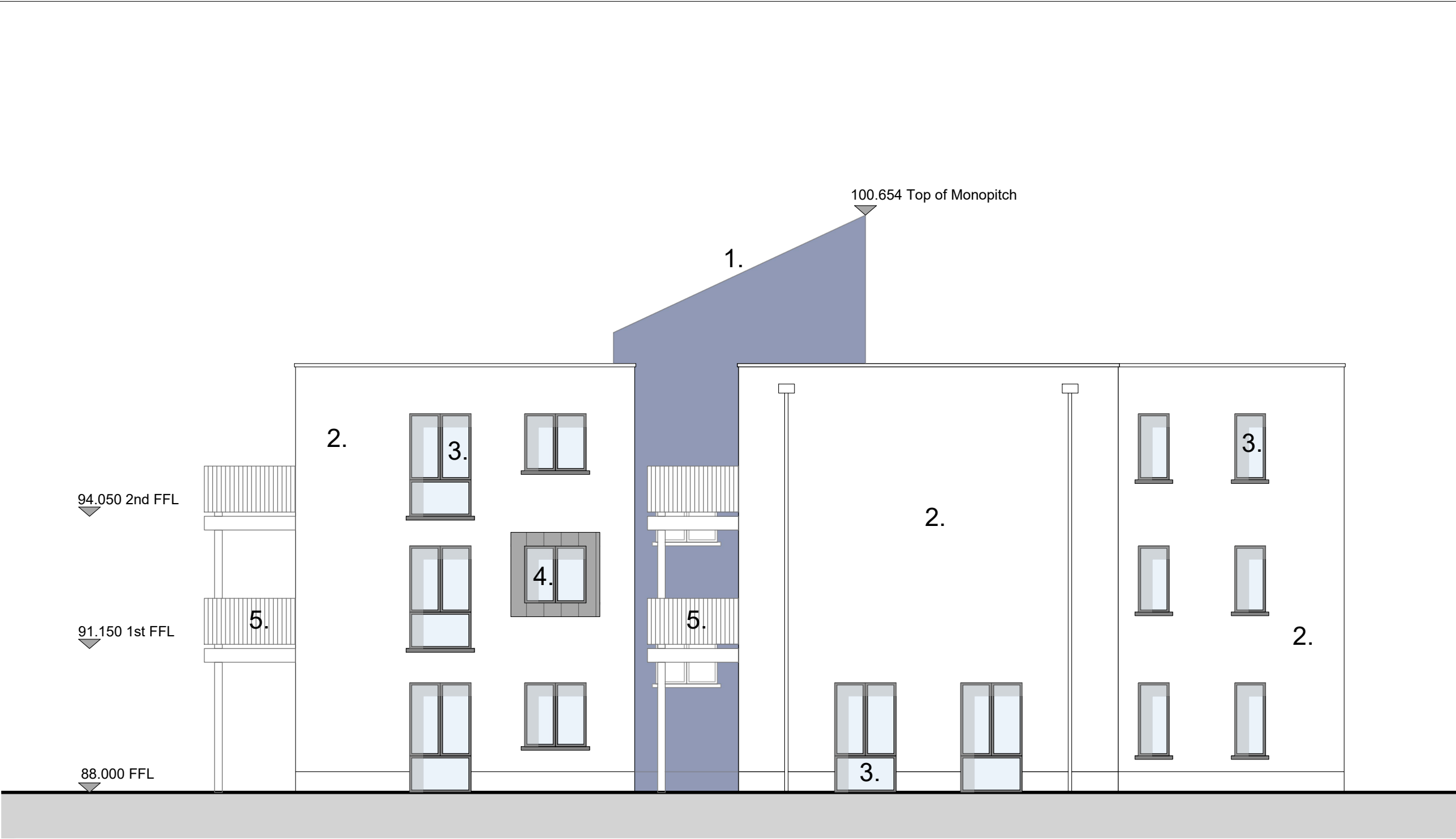
EAST ELEVATION - BLOCK D SCALE 1:100 (A3)
