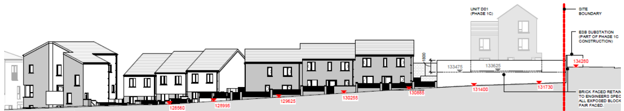
Fig. 5 Phase 3C site section through Aspen Close cul-de-sac showing stepped street elevation and 2.5m high retaining wall at Phase 3C interface (far right, red line marks site boundary)
