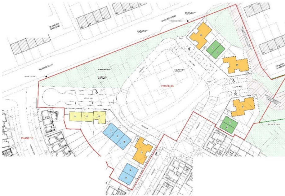
Fig. 3 CNWQR Phase 3C Site Plan, footprint of former terraces shown dashed: proposed 2-storey houses shown yellow & blue, 3-storey houses green, duplex corner blocks orange
