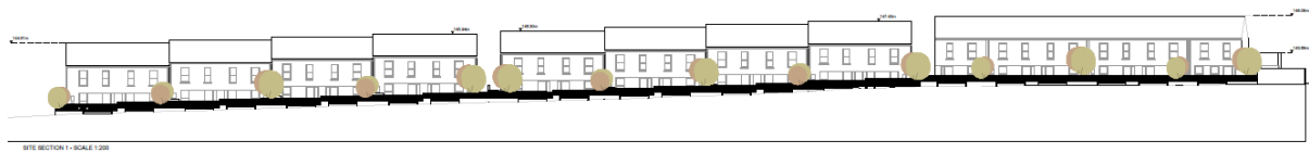
Fig. 5 Phase 4C West site section through new road showing stepped street elevation
