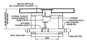
FIRE HYDRANT SECTION (SCALE 1:25)
