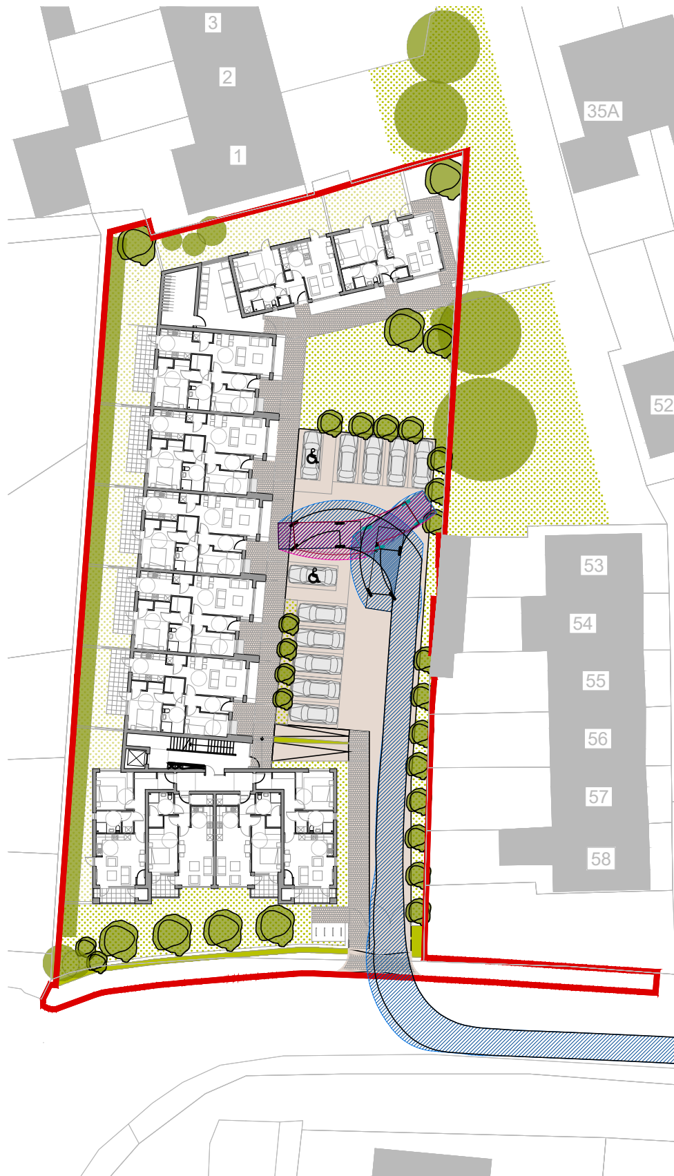
PROPOSED FIRE TRUCK TURNING SCALE 1:250
