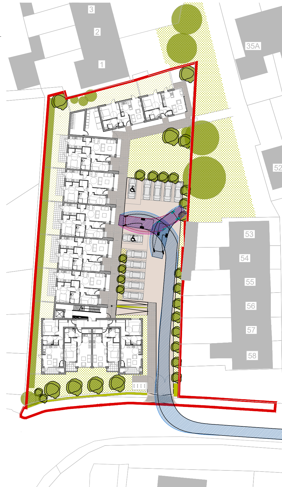
PROPOSED REFUSE TRUCK TURNING SCALE 1:250
