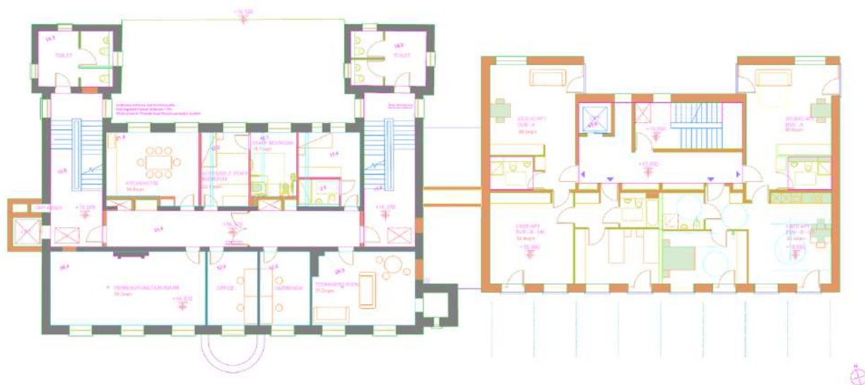
Fig.204: First floor plan of convent building showing proposed additions in orange
