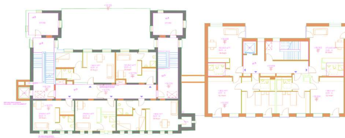
Fig.205: Second floor plan of convent building showing room numbers and showing proposed demolition in blue
