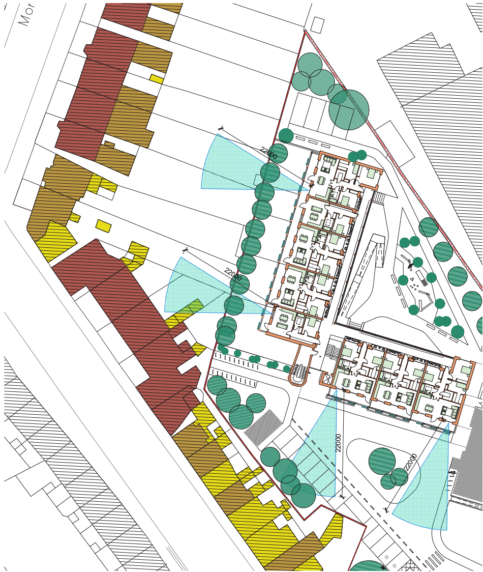
Overlooking Diagram - shows standard 22m separation distance - view cones will now be obscured by the balcony screens
