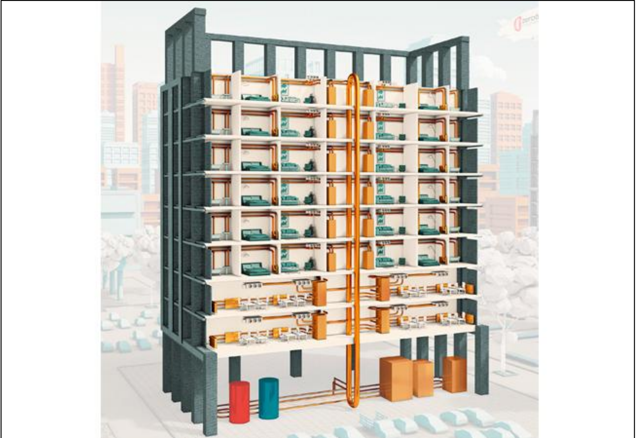
Figure 12: Glendimplex Zeroth Energy System (Ambient Loop)
