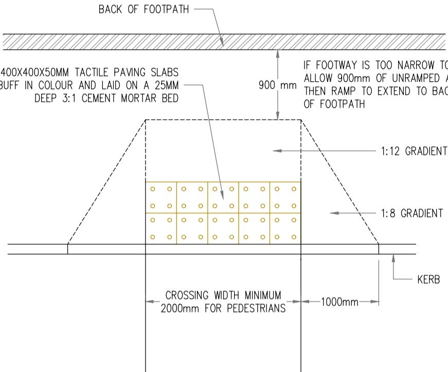
TACTILE PAVING PLAN AT UNCONTROLLED PEDESTRIAN CROSSINGS.
