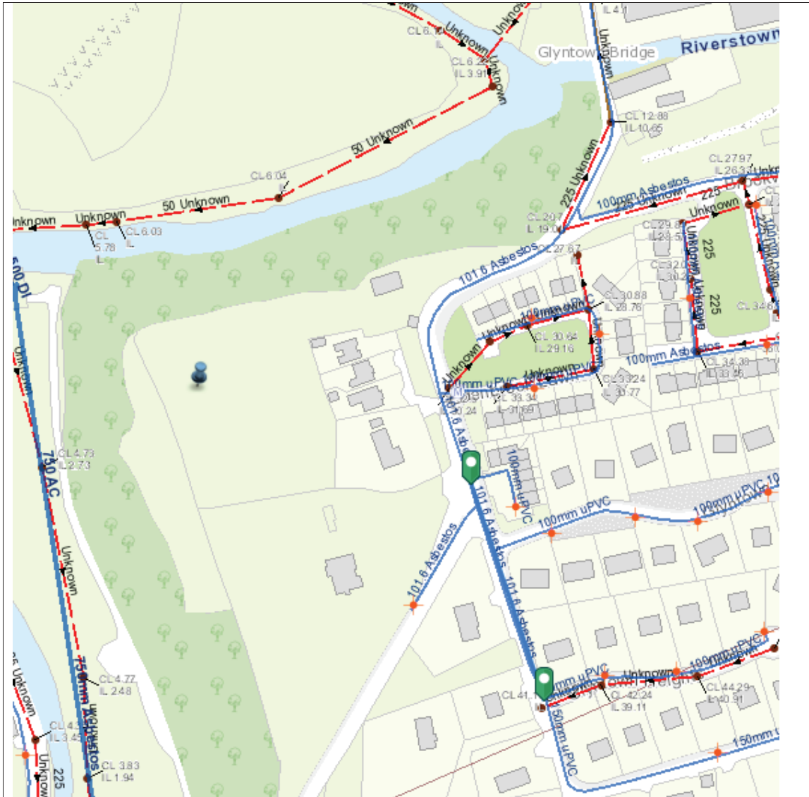
Reproduced from the Ordnance Survey of Ireland by Permission of the Government. License No. 3-3-34
