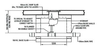
FIRE HYDRANT SECTION (SCALE 1:25)
