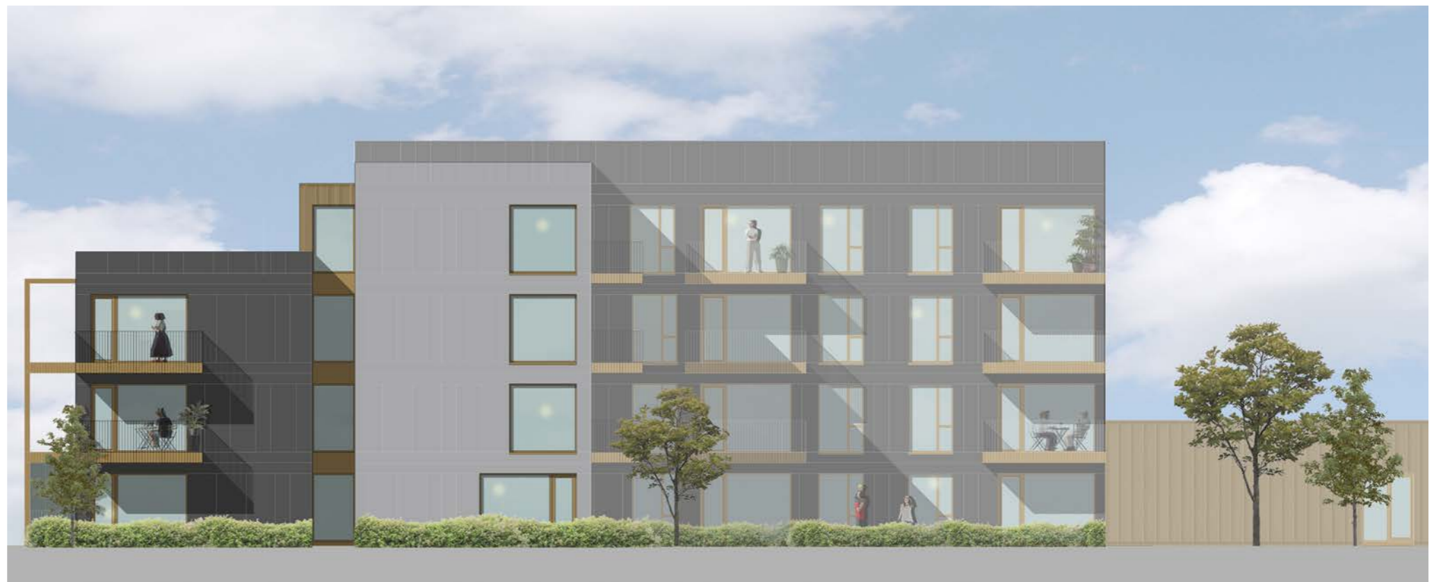
Proposed south elevation Block B showing alternating light and dark grey contrasting fibre cement (or similar) cladding
