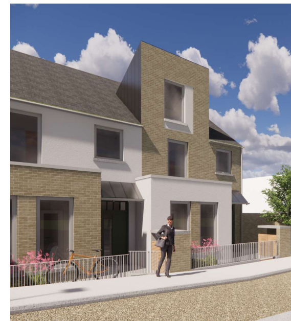
Ground floor apartments include a private space approx. 2.5m deep and enclosed by painted galvanized steel railings. This space incorporates weathered bin storage
