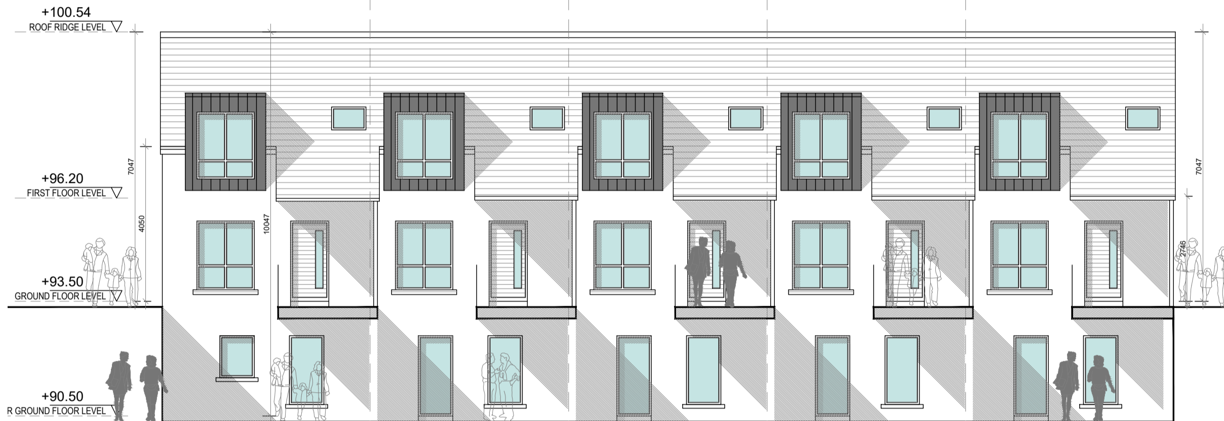
Proposed Front South Elevation - Block C - Terrace of 5 SCALE 1:100 @ A1
