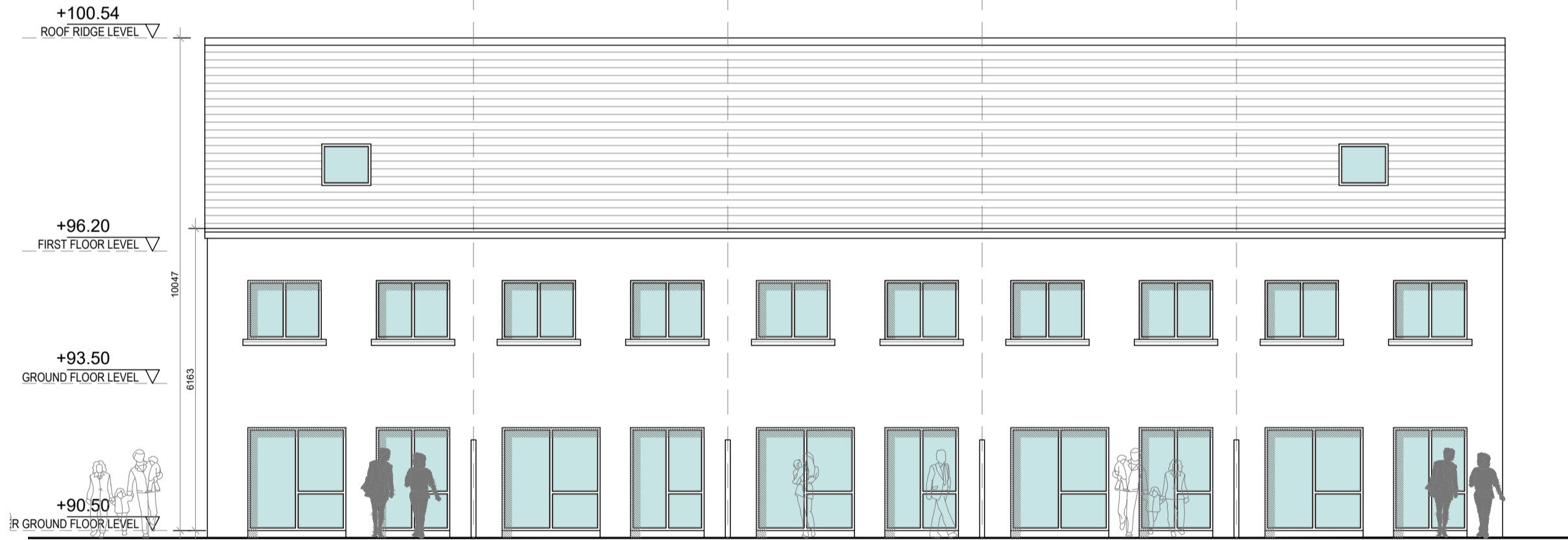
Proposed Rear North Elevation - Block C - Terrace of 5 SCALE 1:100 @ A1
